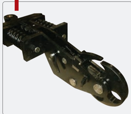
Disc type towing hook with shock absorbers
