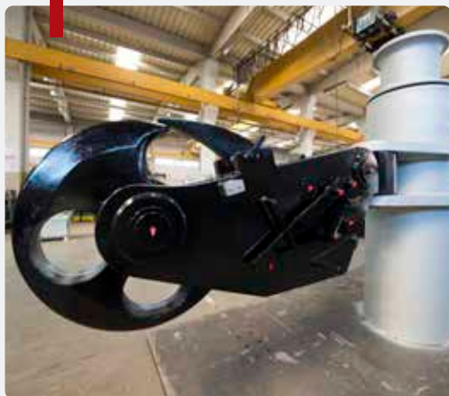
Towing hook foundation with integrated manoeuvring capstan
