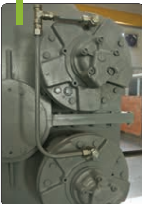
Radial piston type hydraulic motors
