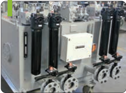
Main engine driven power unit hydraulic tank.
