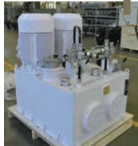
HPU for 2 windlasses with double electric motor
